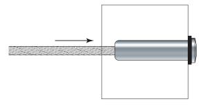
5. Pull cable to set gripping action of the Push-Lock™ Fitting.
