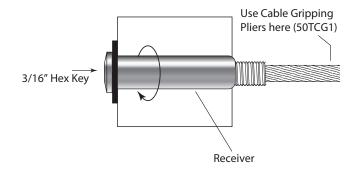
Tension in sequence, beginning with the outside cables and moving from side to side toward the cente
