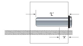
4. Push the cable into the hole in the fitting as far as it will go (approximately 1-1/1\%'s) the cable in the right-hand direction (with the lay of the cable) as you push it into the fittimu will feel it slide through the jaws inside the stud.
