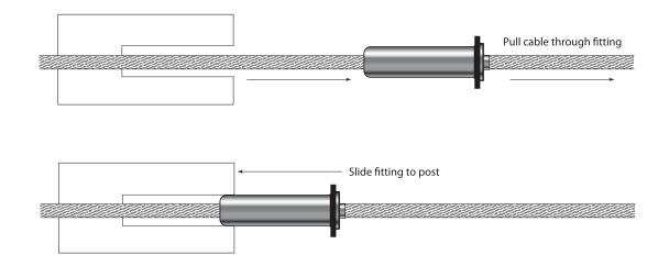
Hold the cable with one hand and slide the Pull-Lock<sup>™</sup> fitting into the hole in the post. Press the back of the fitting to hold it securely in the post and pull the cable through the fitting until it is as tight as you can make it.
