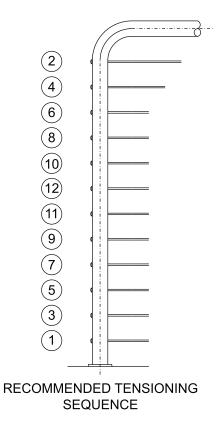
Tension in sequence, beginning with the outside cables and moving from side to side toward the cente
