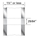
Drill and tap 5/16-24 threaded hole on the inside of the other end post for the Push-Lock fitting.
