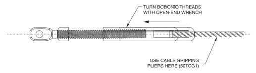
Tension in sequence, beginning with the outside cables and moving from side to side toward the cente
