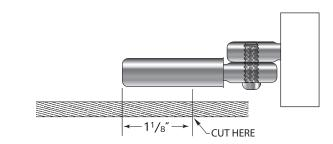
3. Push the cable into the hole in the fitting as far as it will go (approximately 1-1/16"). Twist the cable in the right-hand direction (with the lay of the cable) as you push it into the fitting. You will feel it slide through the jaws inside the stud.
