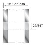
Drill and tap 5/16-24 threaded hole on the inside of the other end post for the Push-Lock fitting.
