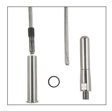
**3.** Start the threaded stud attached to the cable into the Receiver and turn 2 complete turns. This will thread about 1/3 of the stud into the Receiver.
