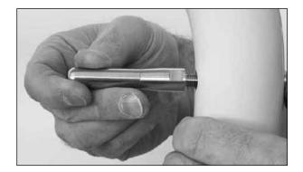
**6.** Thread the Push-Lock coupler onto the post and tighten with 7/16" wrench.
